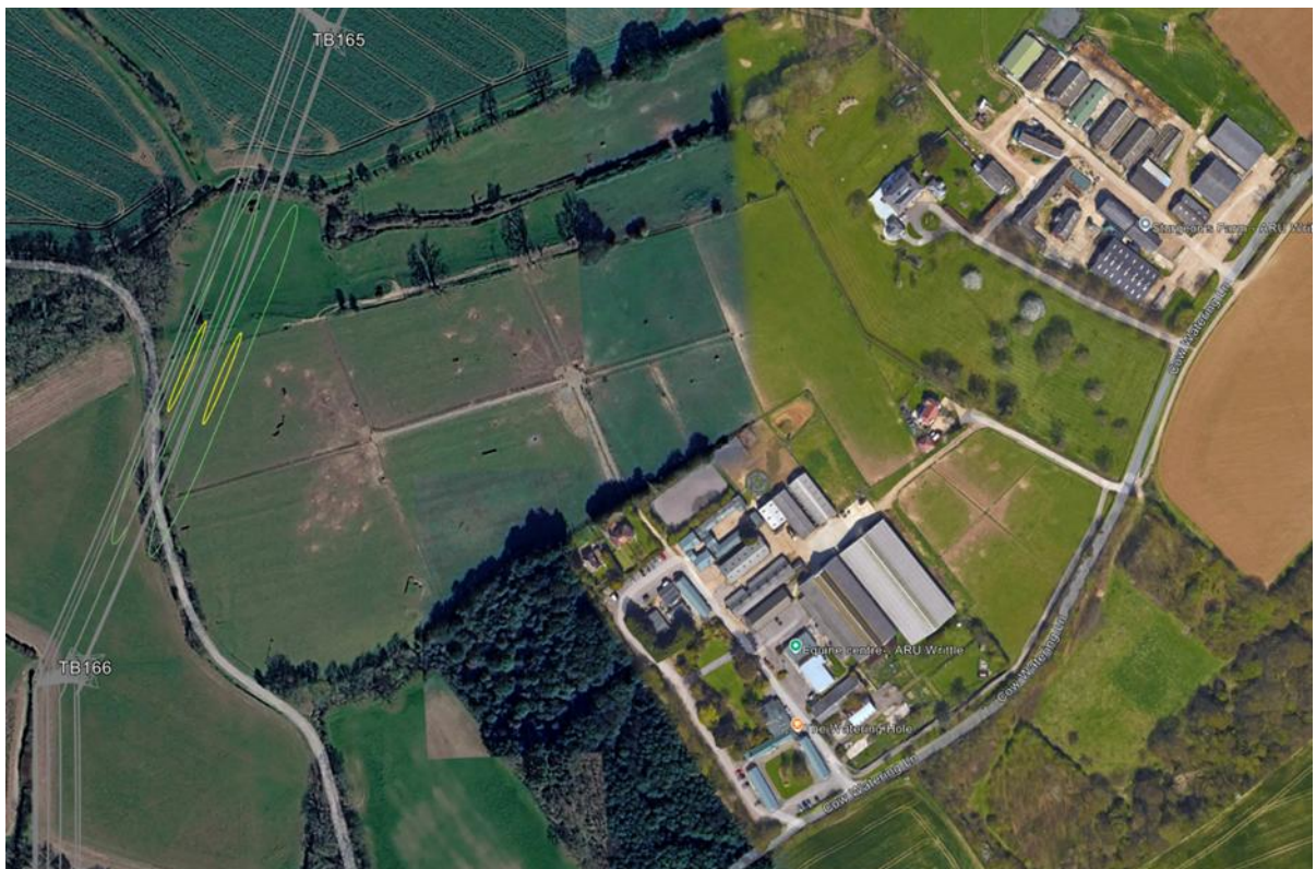
Figure 1 Illustrated maximum calculated electric fields from Spans TB165 to TB166. Yellow contours detail where the electric field would be at its maximum of 2.8 kV/m directly under the conductors and the green contour indicates where the electric field reduces to between 2.8 and 2.0 kV/m.
